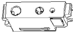
Figure 5: Bottom connector including the microphone
